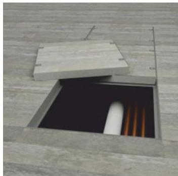
The Floor Access Cover Series 7500 BS multidoor is made of aluminum. The depth of the tank is 62 mm and the height of installation is only 75 mm. The manhole cover is equipped with three special gaskets all around the perimeter. The frame is fixed by throwing at floor level.
